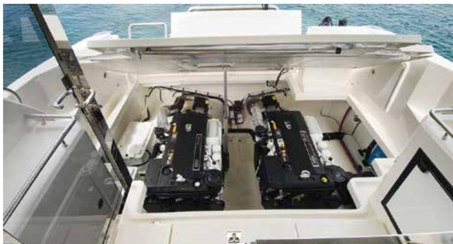
For access to the engine room, nearly the entire cockpit sole opens with the hydraulic hatch lift exposing the Volvo diesel engines. There is plenty of space for fluid checks and service.
