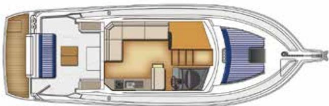
The large cockpit flows into the large combination saloon/galley with the helm station forward and to starboard.
